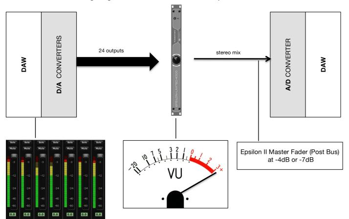
In a "saturated" mix the DAW output levels are "high". Inside our summing bus the signal levels are will be off the scale and the Epsilon master fader requires attenuation. This is the same situation when using an analog console the master vumeters are off scale. The Epsilon requires that the master fader attenuate the output levels to send the mix to DAW or other analog gear.
